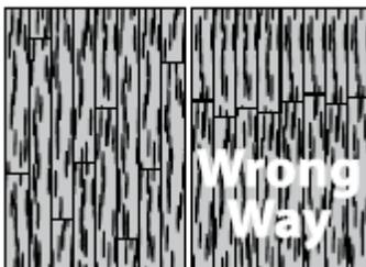
Using the longest pieces available, lay the first row against the longest and straightest wall. Carefully apply glue into top of groove along the whole length of the piece, using glue specially designed for hardwood flooring. Lay the first piece with the grooved
